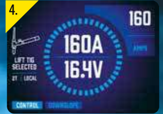
4. LIFT TIG 溶接画面
